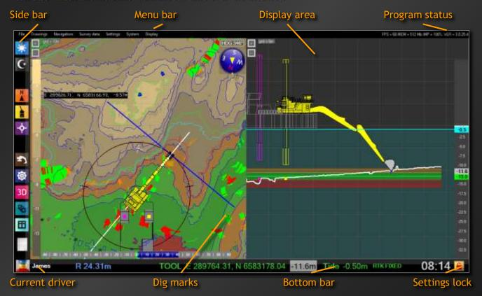
The software is fully configurable to your vessel and equipment setup and can be loaded with AutoCAD drawings and raster maps to accurately depict your machine and the current working area.
